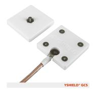
YSHIELD GmbH & Co. KG Rotthofer Straße 1 94099 Ruhstorf, Germany Further information: www.yshield.com, info@yshield.de Grounding connection with two plates that get screwed together. For all electrically conductive fabrics, fleeces, meshes. The two connecting plates must be screwed together - the material that is supposed to be grounded needs therefore to be perforated.
